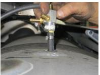
The fuel draw tube is designed to vent the fuel tank as well as supply and return fuel to the APU.
